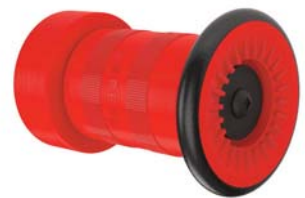
Code 36 Combination Fog Nozzle Material: Polycarbonate Standard Threads: NPSH Sizes: 1 1/2" (75 GPM)
