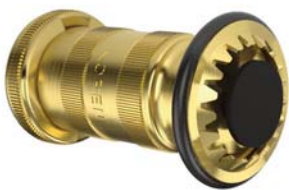
Code 37 Combination Fog Nozzle Material: Brass Standard Threads: NPSH, NST Sizes: 1 1/2" (75 GPM)
